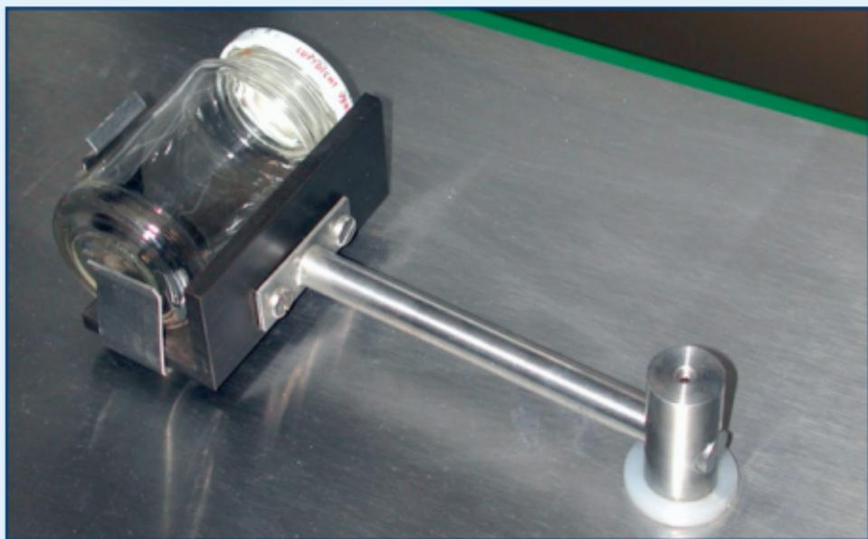
**Friabimat™** used for testing the friability of pellets
