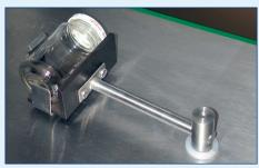
Friabimat™ used for testing the frigbility of pellets
